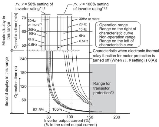
This function detects the overload (overheat) of the motor, stops the operation of the inverter's output transistor, and stops the output. (The operation characteristic is shown on the left.)
